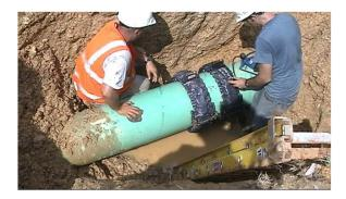
Utilizing Long Range Guidedwave Ultrasonic equipment, the pipe segment between excavations is inspected for anomalies. All anomalies indicated by the GUL inspection are then excavated and examined utilizing our Automated Ultrasonic Corrosion Mapping System (shown to the right). This system provides documented results verifying the existence or nonexistence of internal, mid-wall, or external anomalies. It performs the CORROSION INDUSTRIES INC.
