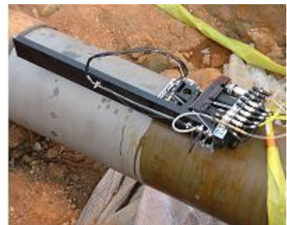
Automated Ultrasonic Corrosion Mapping System
