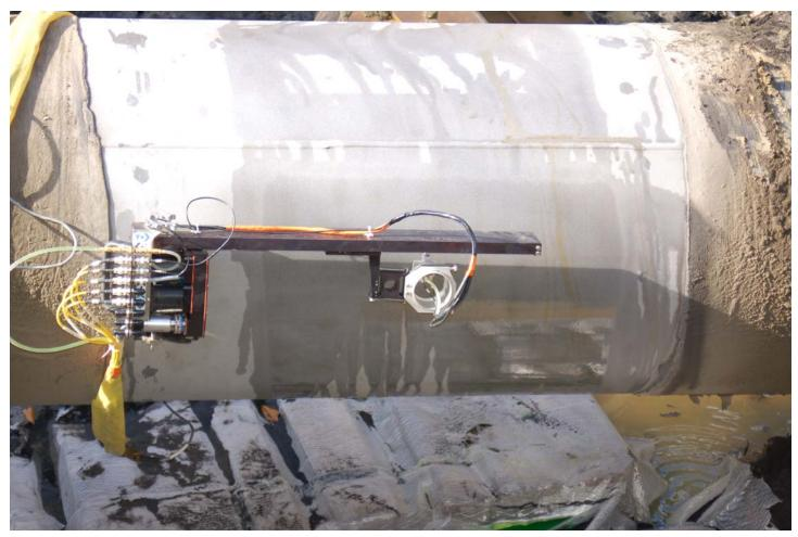
Introducing IntraSpect automated ultrasonic internal & external corrosion mapping system with 5080 robotic pipe scanner:
